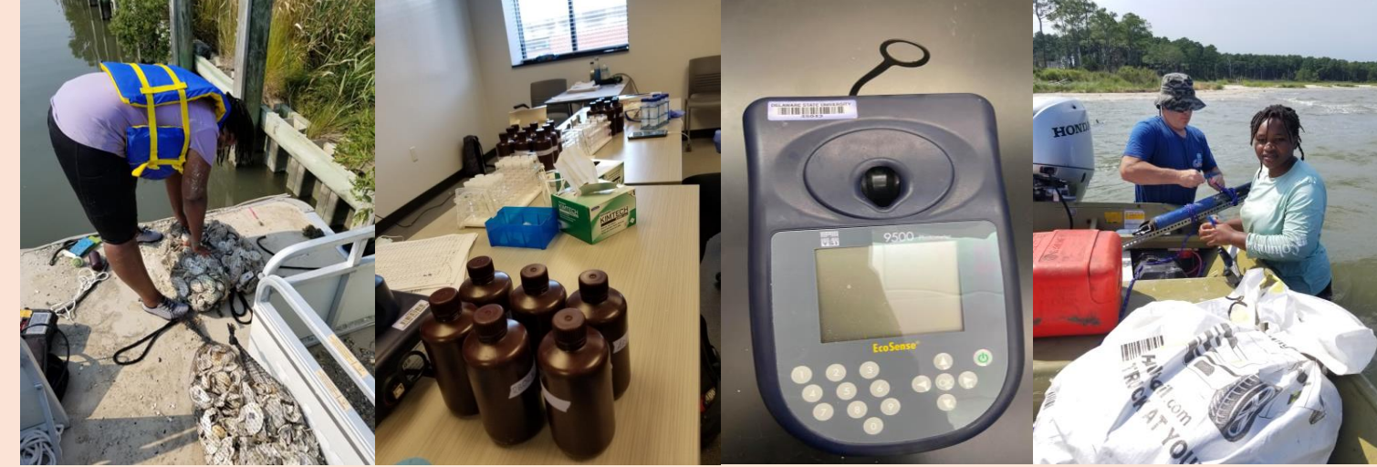
Figure 4 (a-d). Demonstrates a) deployment of oyster shell bags, b) chemical water quality testing, c) YSI 9500 Photometer, d) YSI EXO sonde deployment
