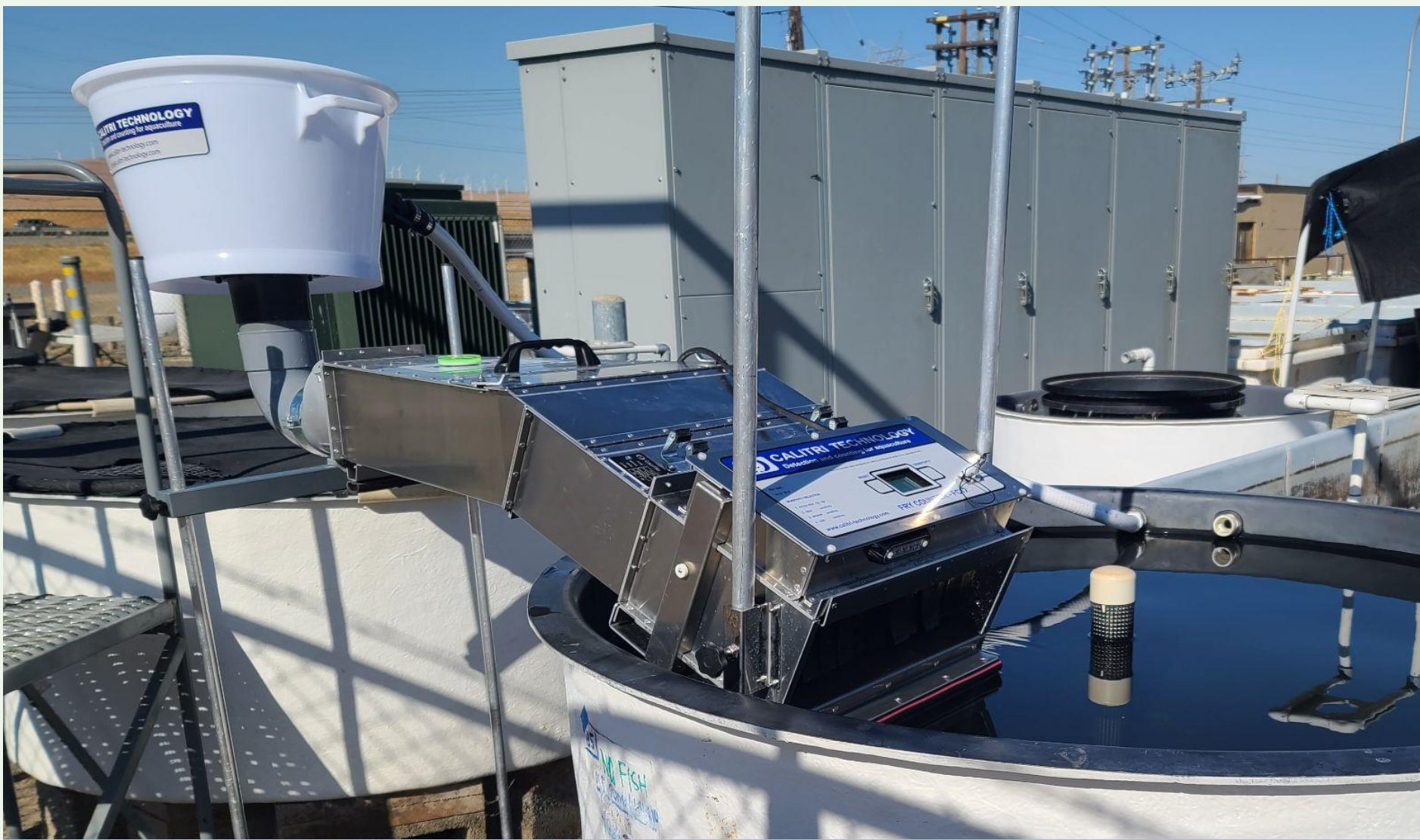
Figure 1. An FC12 Fry Counter (Calitri Technology, Walcourt, Belgium) was used for the study. The device was connected to a white loading tank with its central fish absorber removed and set up for manual operation.
