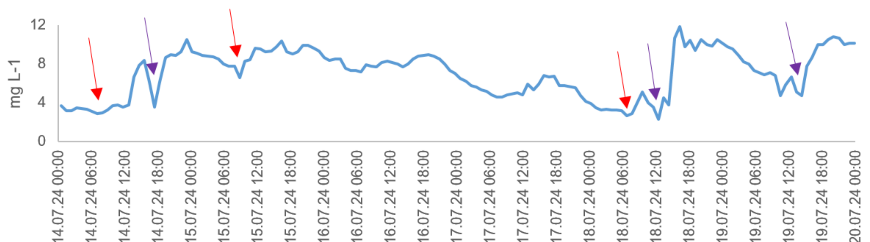
Fig. 5: Shows the DO between 14.7. – 19.7.2024. Red arrows mark the lowest concentrations in the early morning hours, which is common due to photosynthetic activity of algae and plants. Purple arrows mark the effect of the aeration (mixing the layers lowers the DO at the surface, if there is an extreme low DO content in deep layers).
